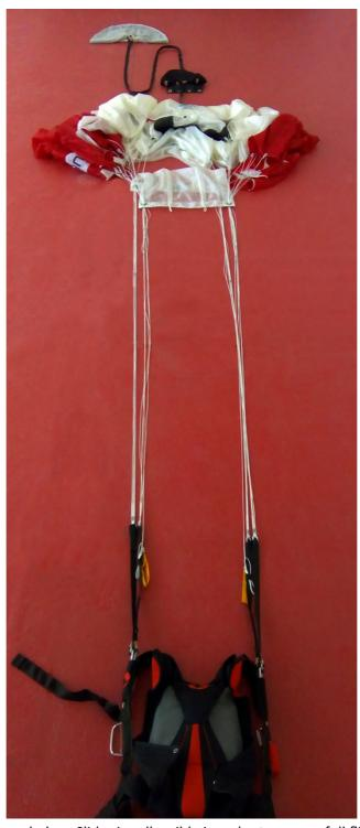
Stretch the slider as shown below. Slider is collapsible in order to ensure full flight performance, avoid
