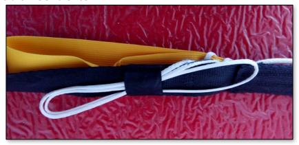
Brake set and secured for packing/jump.
